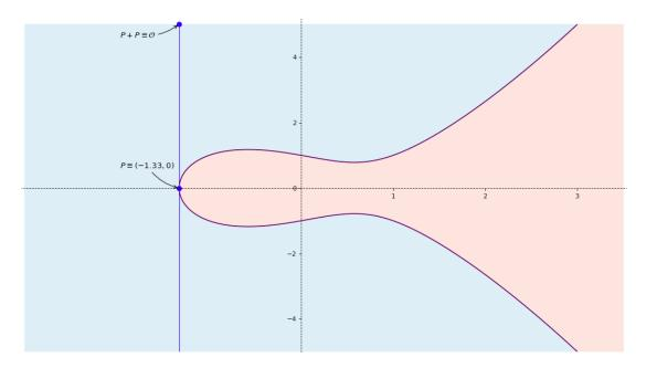
Configuration #4: The two points on the elliptic curve are identical and constitute an inflection point. We let the point be denoted by  $P \equiv (x_p, y_p)$ .
